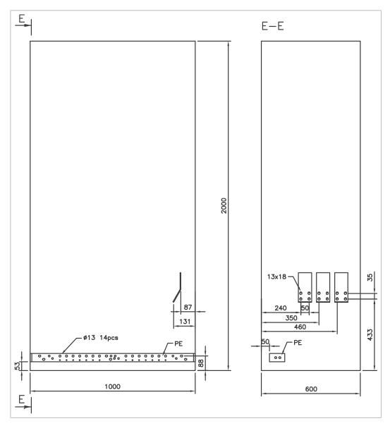
Sine filter cubicle, 1000 mm, bottom cable exit
