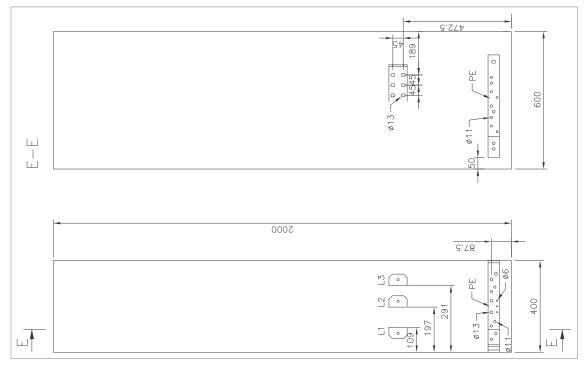
Frame 2×R8i+2×R8i with main switch/disconnector (400 mm), bottom cable entry (+H353)
