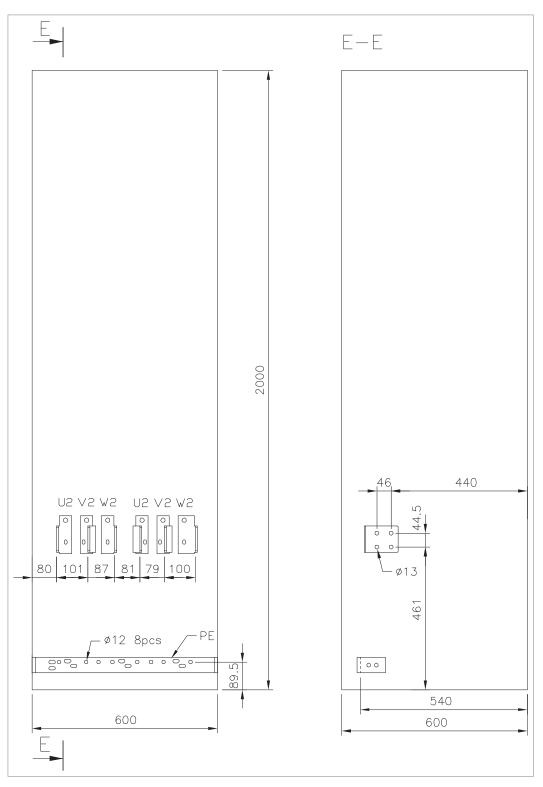
Inverter module cubicle with two R8i modules, bottom cable exit
