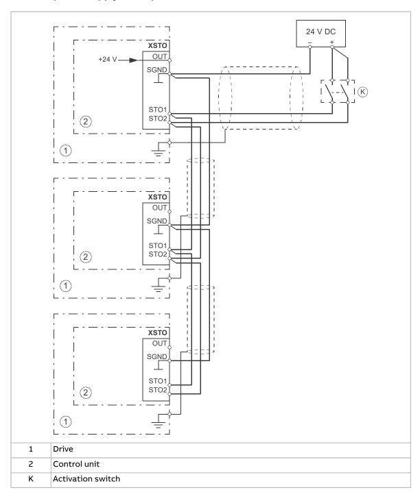
External power supply (example, drives with UCU-2x)
