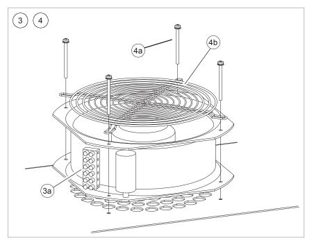
Replacing a roof fan (IP54/UL type 12)
