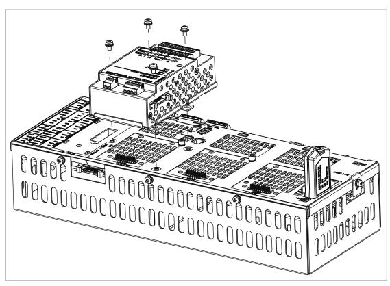
3. Attach the FSO module onto slot 3 of the BCU control unit [A41] with four screws.
