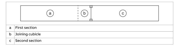
4. Attach the front and rear posts of the joining cubicle to the posts of the other section with 16 screws (8 per post). Tighten the screws to 5 N·m (3.7 lbf·ft).
