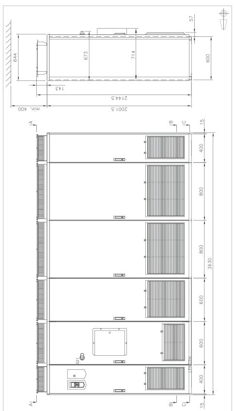
Frame 3×R8i+3×R8i with common motor terminal cubicle (+H359), 1/2
