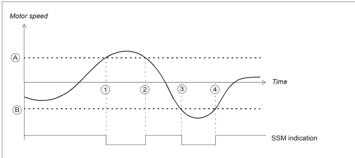
A SSM1 limit positive (parameter *SSMx.13*)
