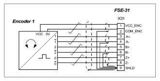
**Note**: This diagram is applicable to all revisions of FSE-31. But the voltage for VCC is:
