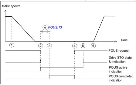
POUS delay for completion (parameter POUS.13): Sets a delay for POUS completed indication. The POUS completed indication (parameter POUS.22) goes on after this delay.
