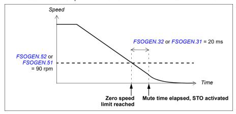
**Example 2**: Zero speed limit is reached with the SS1 function (or SSE with emergency ramp), a negative SBC delay (parameter SBC.12 STO SBC delay) is configured in the STO function:
