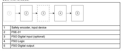
Safe speed monitor (SSM) with encoder includes the following subsystems: safety encoder (not provided by ABB), FSE-31, FSO Digital input (optional), FSO Logic, and FSO Digital output.
