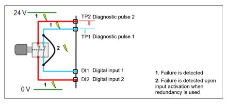
**Note**: If only one of the redundant inputs is activated upon a safety function request, the FSO module activates the safety function in which the input is configured but it cannot be acknowledged before the failure has been repaired. To acknowledge the safety function, you must set both input channels down and up at the same time or, switch the power off and on.
