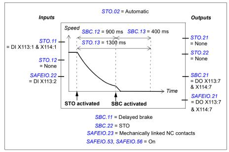
**Example 2 (with an encoder):** The figure below shows an example of the SBC after the STO function set-up when an encoder is used. Configure the safety encoder interface first (see section *Configuring the safety encoder interface* on page 315).
