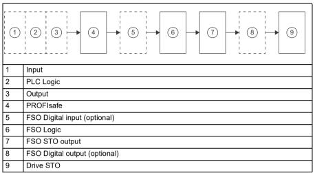
PROFIsafe can replace digital inputs and/or digital outputs of the FSO. For example, it is possible to use PROFIsafe input and FSO output in the same configuration.
