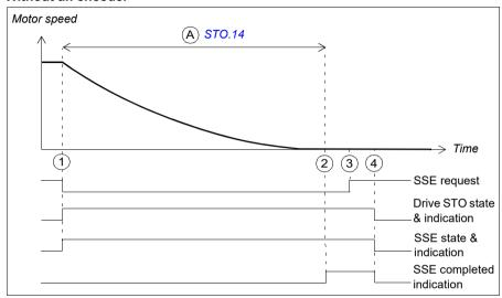
A Time to zero speed (parameter *STO.14*): Time from the STO activation to the moment when the safety function is completed, the SSE completed indication (parameter *SSE.22*) goes on and the acknowledgment becomes allowed. You must set this to the estimated time in which the motor coasts to a stop from the maximum speed.
