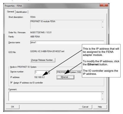
Note: Do not change the IP address assigned here. Use the same IP address for the FENA adapter module also in other tools (eq. the Drive Composer pro PC tool) which you use to connect to the drive.
