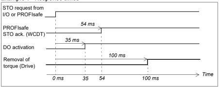
Note: The values shown above are applicable to ACS880 drives. The maximum response time for DCS880 drives is 550 ms.
