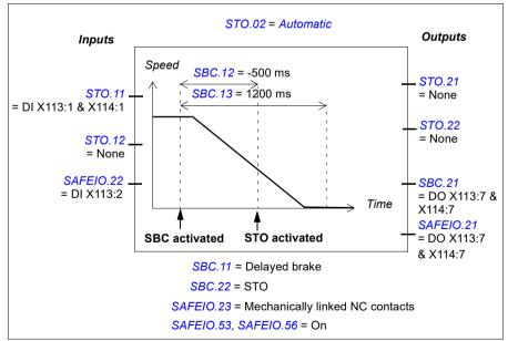
**Example 2 (with an encoder):** The figure below shows an example of the SBC before the STO set-up when an encoder is used. Configure the safety encoder interface first (see section *Configuring the safety encoder interface* on page 315).
