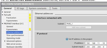
10. In Ethernet addresses submenu, set the PLC IP address.
