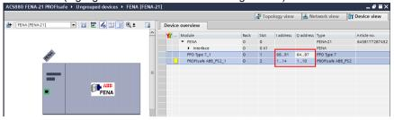
Select PLC from network view and Properties will show on the bottom of the screen. In PLC properties, enable F-capability (safety and PROFIsafe) under the Fail-safe submenu.
