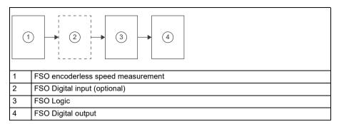
Encoderless SSM includes the following subsystems: FSO encoderless speed measurement, FSO Digital input (optional), FSO Logic, and FSO Digital output.
