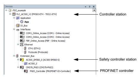
6. Right-click on the PROFINET controller CM579-PNIO-Master and add the FENA module to the PROFINET IO network.
