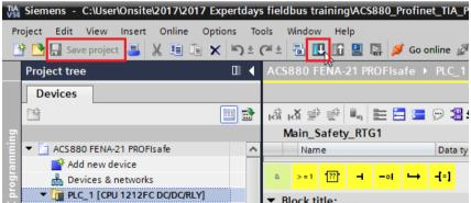
25. Scan for accessible devices (start search). Note that a firewall can block traffic.
