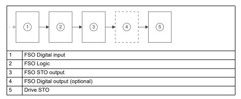
Prevention of unexpected start-up (POUS) includes the following subsystems: FSO Digital input, FSO Logic, FSO STO output, FSO Digital output (optional), and Drive STO
