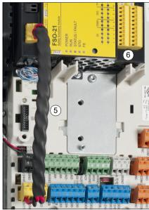
7. Connect the power supply wires to the FSO terminal X112. Use a tightening torque of 0.24 Nm (2.1 lbf·in) for the FSO terminals. Use proper cable strain relief. See also section Power supply connection/cables on page 291.
