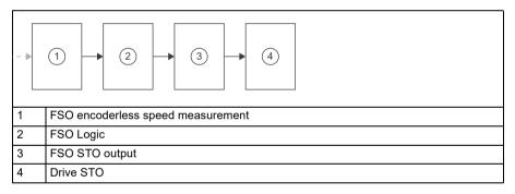
Safe maximum speed (SMS) includes the following subsystems: FSO encoderless speed measurement, FSO Logic, FSO STO output, and Drive STO.
