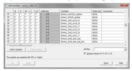
**Note**: In PROFINET communication, the bits of each octet are sent the most significant bit first. Therefore, the bits of every octet in the PROFINET message are in reversed order compared to the bits shown in the figure. For example, the first bit that is sent in the PROFINET message is the 7th bit of the first octet (I 0.7).
