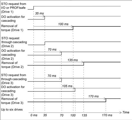
Note: The values shown above are applicable to ACS880 drives. The maximum response time for DCS880 drives is 550 ms.
