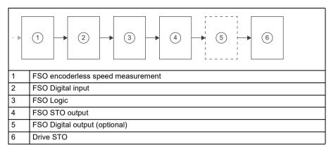
Safely-limited speed (SLS) without encoder includes the following subsystems: FSO encoderless speed measurement, FSO Digital input, FSO Logic, FSO STO output, FSO digital output (optional), and Drive STO. Block diagram is equal to SS1-r function.
