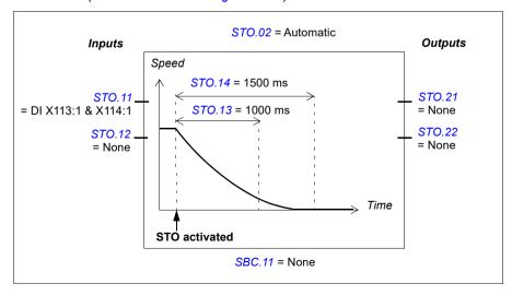
**Example 2 (with an encoder):** The figure below shows an example of a simple STO function set-up when an encoder is used. Configure the safety encoder interface first (see section *Configuring the safety encoder interface* on page 315).
