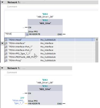
The value can be verified from the HW configuration, in the FENA PPO type properties, under the **Hardware Identifier** tab.
