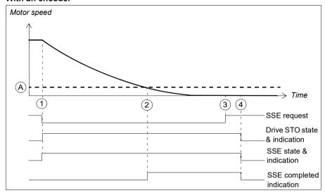
Α Zero speed with encoder (parameter FSOGEN.52): Speed limit at which the motor has stopped, the safety function is completed and the SSE completed indication (parameter SSE.22) goes on. The acknowledgment becomes allowed.
