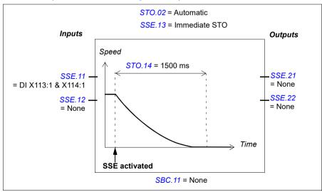
**Example 2 (with an encoder):** The figure below shows an example of the SSE function with immediate STO set-up when an encoder is used. Configure the safety encoder interface first (see section *Configuring the safety encoder interface* on page *315*).
