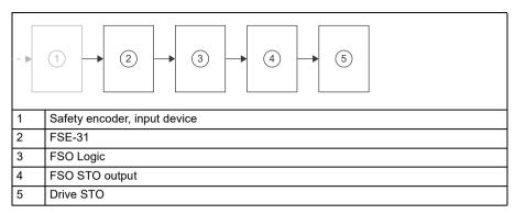
Safe maximum speed (SMS) includes the following subsystems: safety encoder (not provided by ABB), FSE-31, FSO Logic, FSO STO output, and Drive STO.
