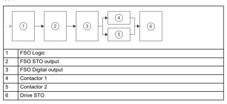
Safe brake control (SBC) includes the following subsystems: FSO Logic, FSO STO output, FSO Digital output, Contactor 1 and 2 (can be provided by ABB), and Drive STO.
