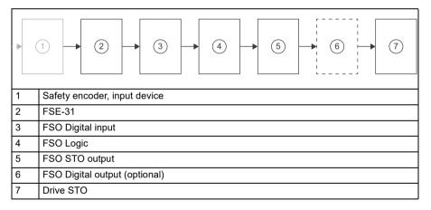
Safely-limited speed (SLS) with encoder includes the following subsystems: safety encoder (not provided by ABB), FSE-31, FSO Digital input, FSO Logic, FSO STO output, FSO Digital output (optional), and Drive STO. Block diagram is equal to SDI and SS1-r.
