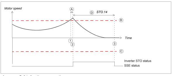
This time scheme diagram illustrates the operation of the SMS function (version 1).
