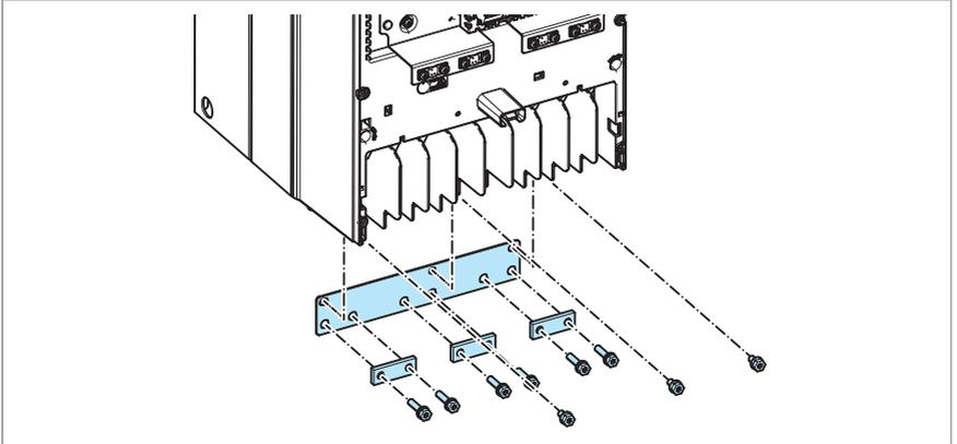
3. Connect the twisted shields of the power cables under the grounding clamps or with cable lugs under the clamp screws.
