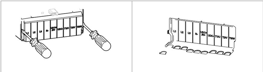
2. Attach the power cable shield grounding shelf to the drive module.
