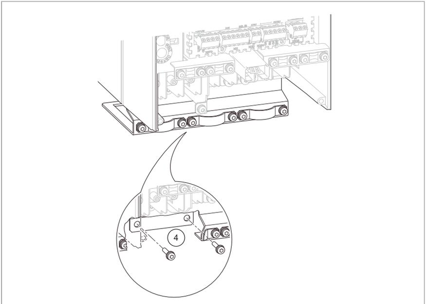
5. Connect the twisted shields of the power cables to the grounding terminals.
