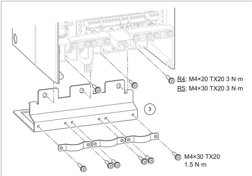
4. Attach the mechanical support shelf for the power cables to the mounting plate.
