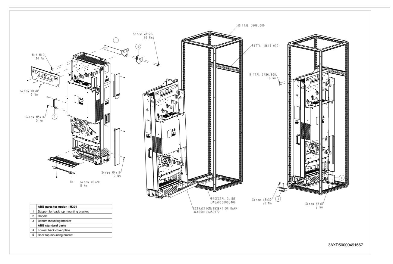
272 Step-by-step drawings for option +H391 installation example in a Rittal VX25 600 mm wide enclosure
