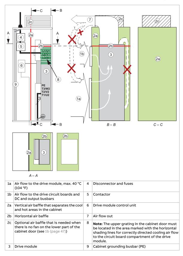
52 Guidelines for planning the mechanical installation
