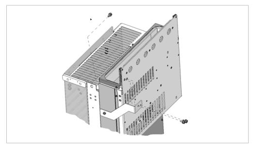
7. Connect the busbars of the drive module to the busbars of the cabling panels (M12 combi screw, 70 N·m [52 lbf·ft]).
