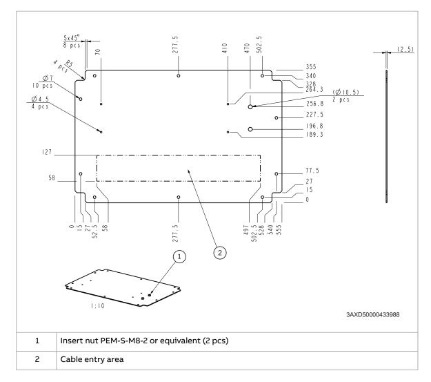
Note: The bottom plate is not an ABB part.
