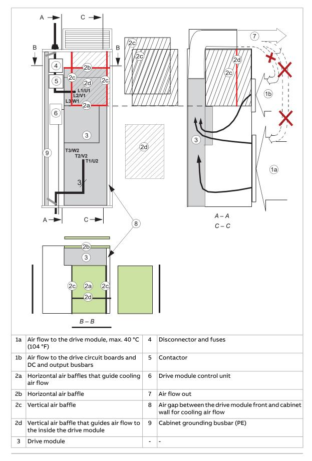
56 Guidelines for planning the mechanical installation
