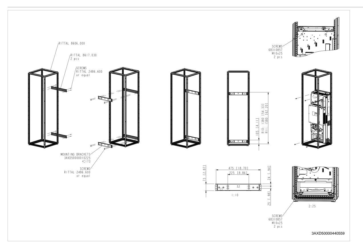
270 Step-by-step drawings for a flat installation example in a Rittal VX25 600 mm wide enclosure
