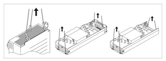
Make sure that the module does not topple over when you move it on the floor: To open the support legs, press each leg a little down (1, 2) and turn it aside. Whenever possible attach the module also with chains. Do not tilt the module. It is heavy and its center of gravity is high. The module overturns from a sideways tilt of 5 degrees. Do not leave the module unattended on a sloping floor.
