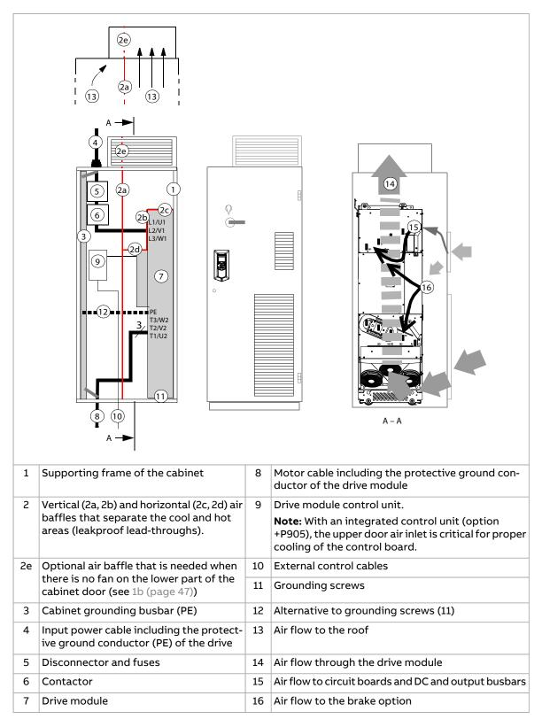
**Note:** The power cable shields can also be grounded to the drive module grounding terminals.
