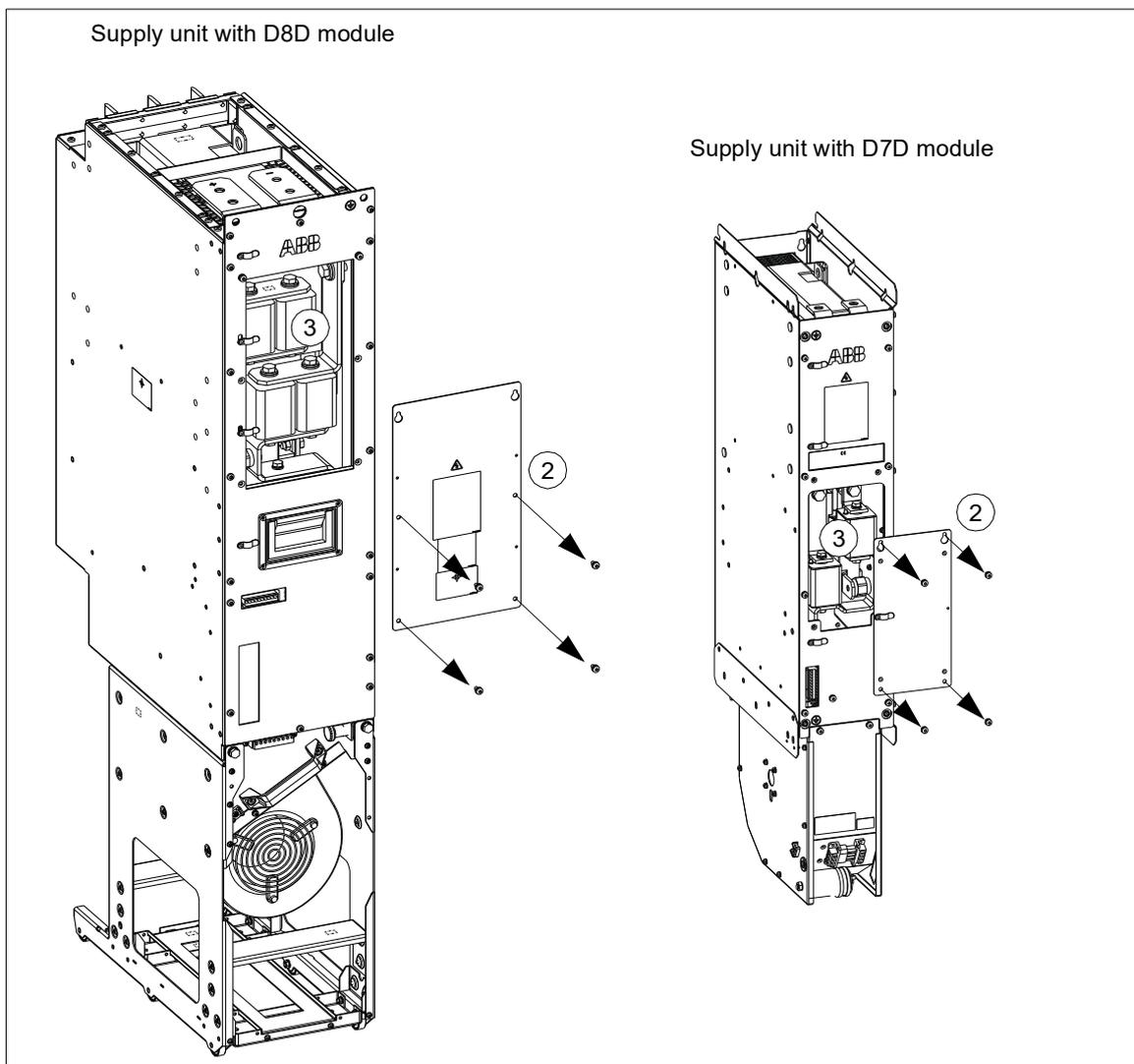
**Note:** The illustration above shows a D8D (IEC) module, which has two fuses connected in parallel for each DC busbar. D8D modules for UL/CSA (with options +C129 and +C134) have a different type of fuse and only one fuse for each DC busbar.
