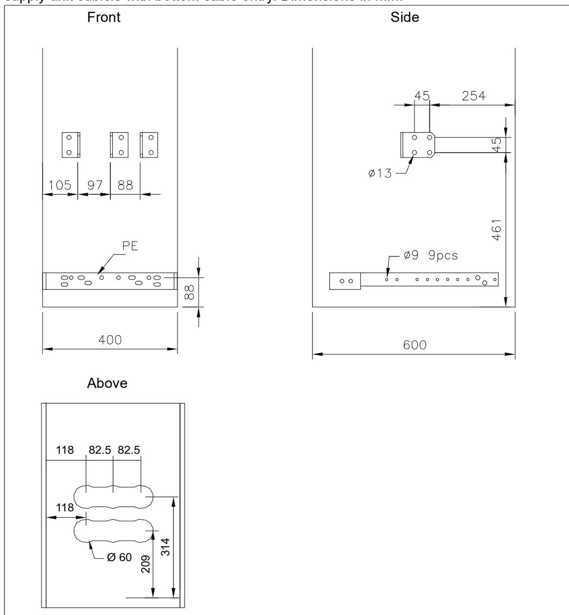
**700 mm supply unit cubicle, bottom cable entry**
