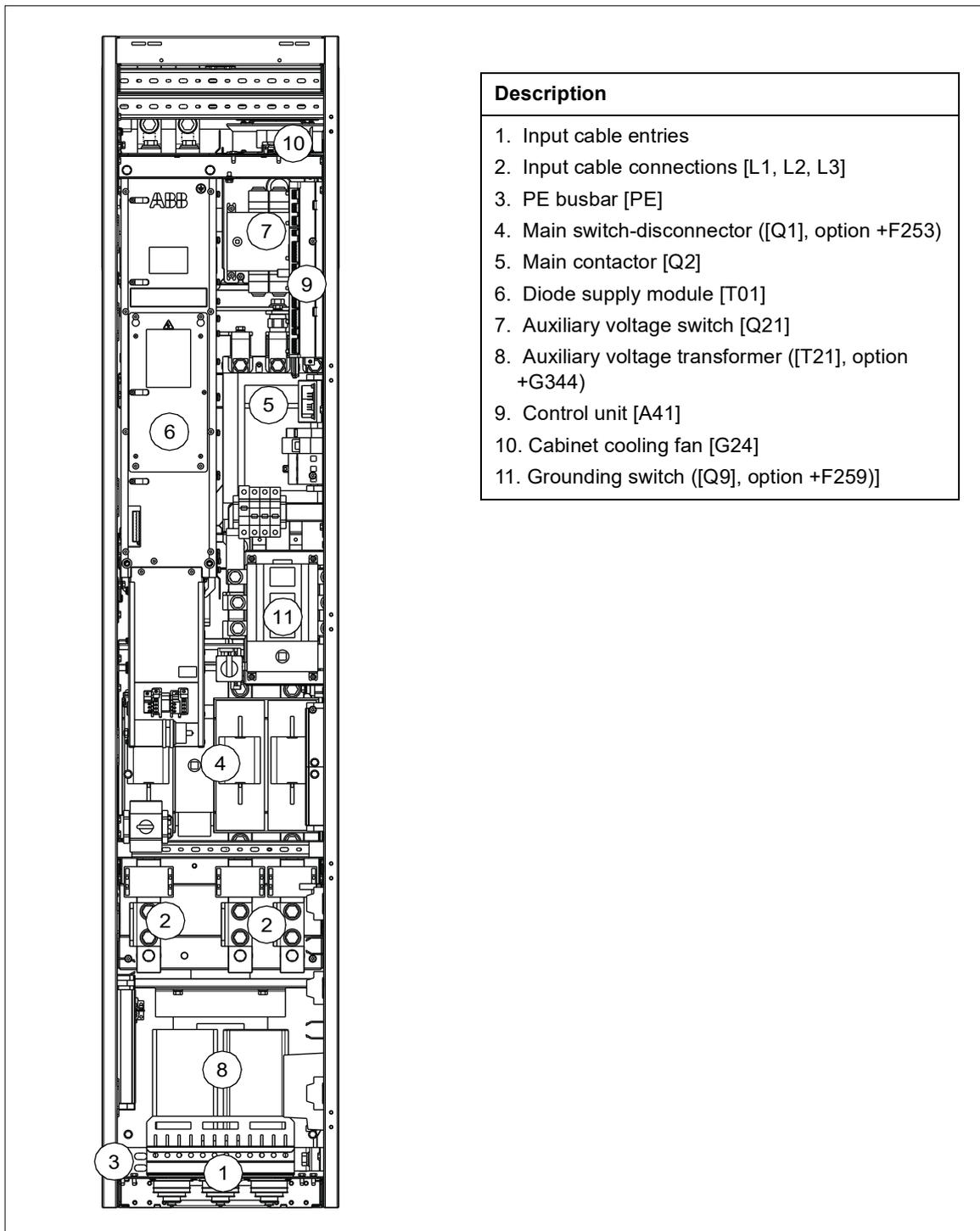
■ **Supply unit with the D8D supply module**
