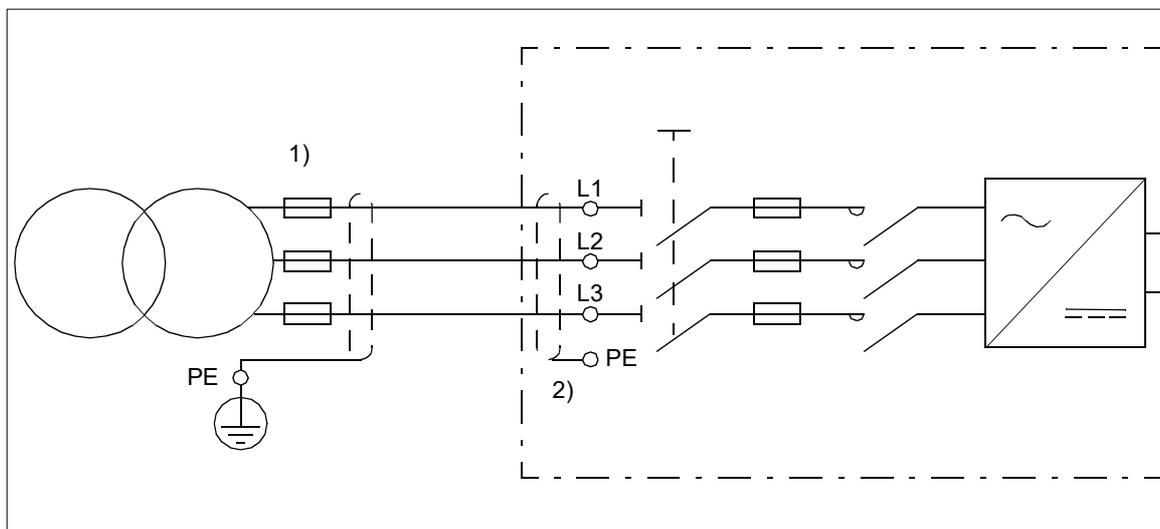
1) Fuses or other protection means. Always use fuses for the cabling of the supply unit with D6D or D7D supply module. See section [Short-circuit withstand strength](#) on page 87.
