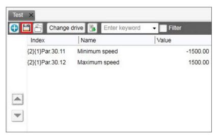
Drive Composer saves to file the values in the **Offline value** column. If the **Offline value** column was empty, then values in the **Values** column is saved.
