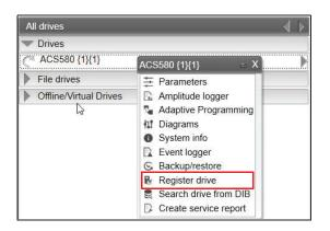
If you used the drive context menu, make sure that Drive Composer is connected online with the drive for successfully registering the drive. If you used **Tools**  $\rightarrow$  **Register drive**, you can register the drive when Drive Composer is either in online/offline mode with the drive.
