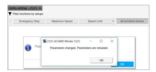
5. Click **OK**, to confirm the password change. You can test the new password, for example, to log in to FSO module (see section, Continue from step 3 in section Printing the safety functions configuration report (Online) (page 146), page 152.) or to read FSO drive parameters (see section, Reading FSO module parameters).
