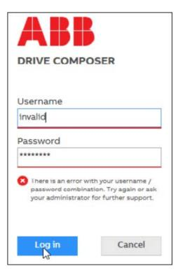
**Note:** Login is successful only when the credentials of drive match with that of RADIUS server. If the credentials are not matching, you may have to shut down the RADIUS server and login to the drive using offline credentials (i.e. service user access level). For default offline credentials, contact your local ABB representative. If login was successful:
