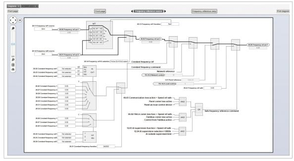
To navigate back to the top level of a Control Diagram, click the **Diagrams top** icon. To navigate through the reference chain, click the buttons circled in the figure above.
