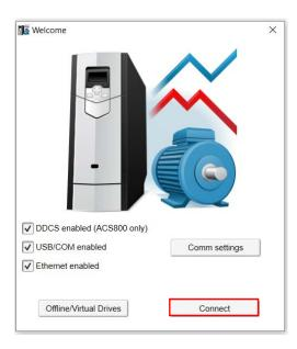
**Note:** If drive is connected via a USB cable, Drive Composer automatically discovers the drive.
