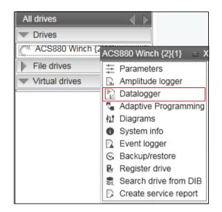
The data collecting can be stopped with a specific stop command or automatically when a triggering condition is true in the drive. After data collection stops you can read and study the data in Drive Composer pro.
