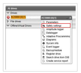
In online mode with FSO installed, the safety configuration already available in the drive is displayed (see figure below). In offline mode the view is always empty before opening the safety file.
