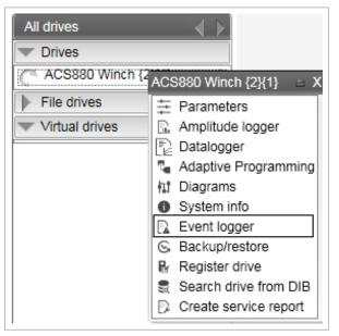
The event logs of the connected drive appears in a separate tab.
