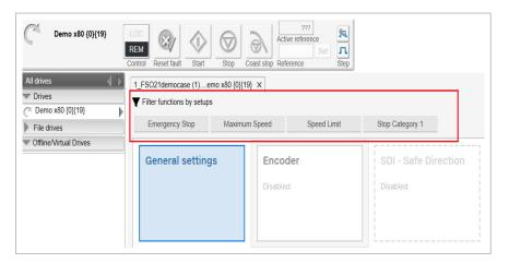
7. In the Graphical view, double-click to open the function. Use the slider switch to enable or disable a function.
