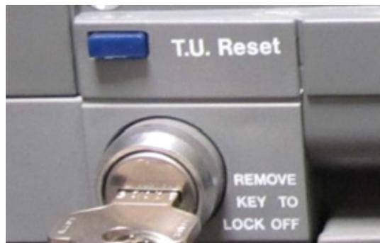
When MCB TRIP appears for the first time, there is a speed warning following MCB TRIP fault in the fault logger of the rotor-side converter. If the PLC continues making automatic reset trials after MCB TRIP and TU-TRIP button is out, the fault logger will fill up with MCB TRIP indications and speed warning is not shown anymore.
