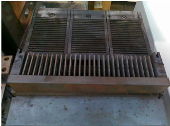
*Heavy signs of short circuit current - The circuit breaker must be replaced*
