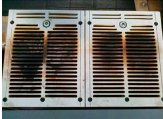
*Medium signs of high current in arcing chambers - No need to replace the circuit breaker*
