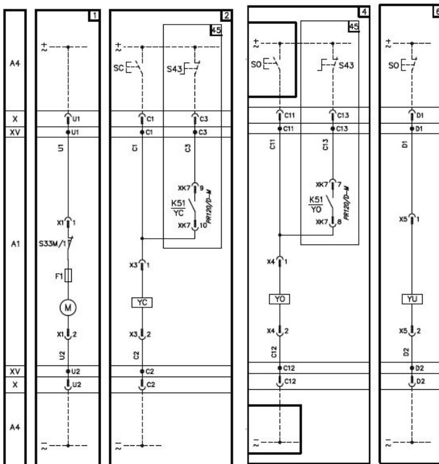
Circuit breaker status is shown in OPEN POSITION, CONNECTED into the cradle, springs discharged.
