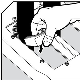
Mount the modules by sliding them in through the angled entry side of the frame.
