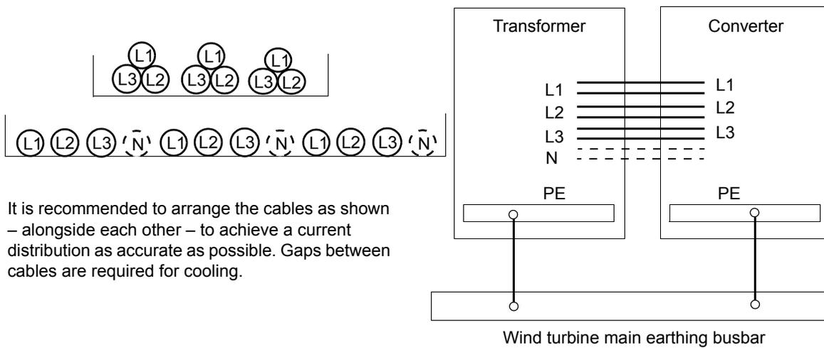
**Note:** Current derating of the cables is required when installing the cables in a cable tray. This derating factor must be taken into account as per the local electrical safety code.
