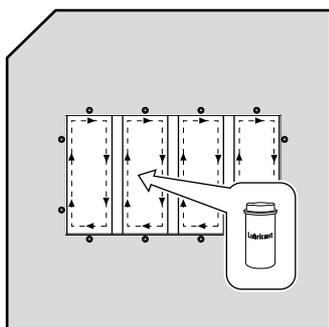
*Lubricate the inside of all frame openings thoroughly with lubricant.*
