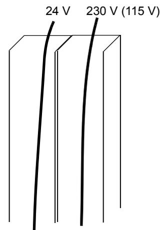
Lead 24 V and 230 V (115 V) control cables in separate ducts inside the cabinet.
