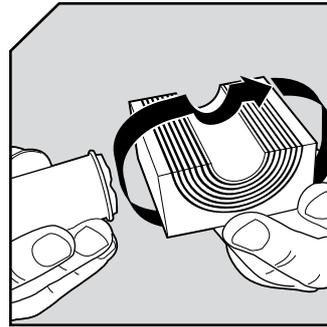
Lubricate all modules for the frame thoroughly on both the inside and the outside surfaces.
