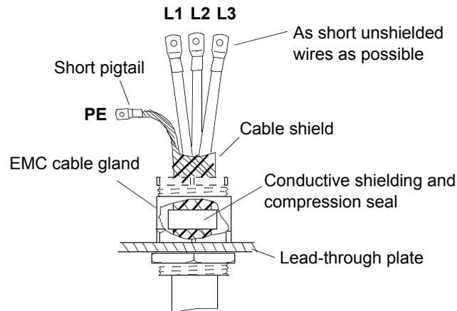
**Note:** EMC cable glands are not included in the delivery. They must be supplied by the customer.
