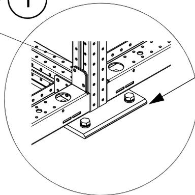
Use M10 or M12 screws; welding is not recommended (see [Electric welding](#) on page 51).
