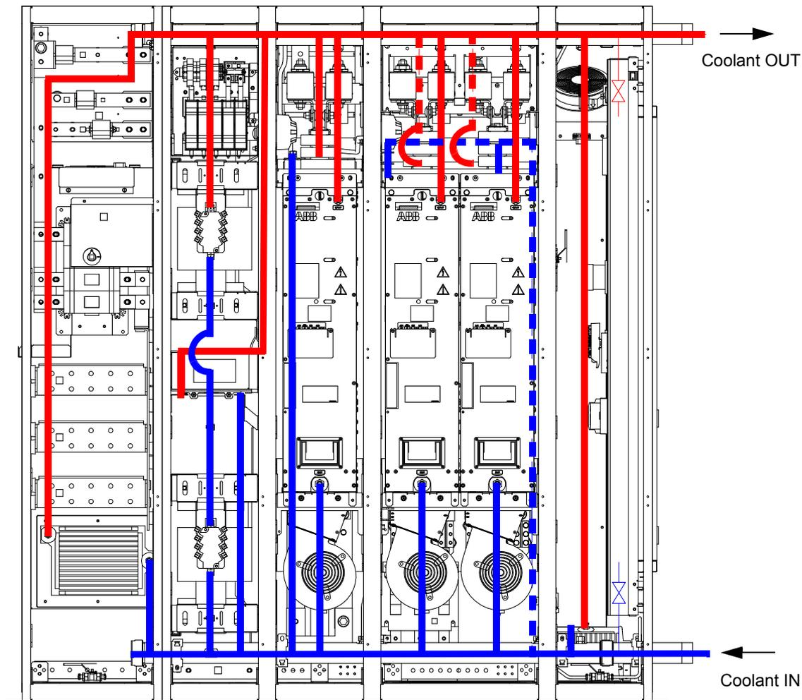
The power modules in each cubicle can not be isolated from the main cooling circuit. The converter is equipped with a drain valve and a bleed valve.
