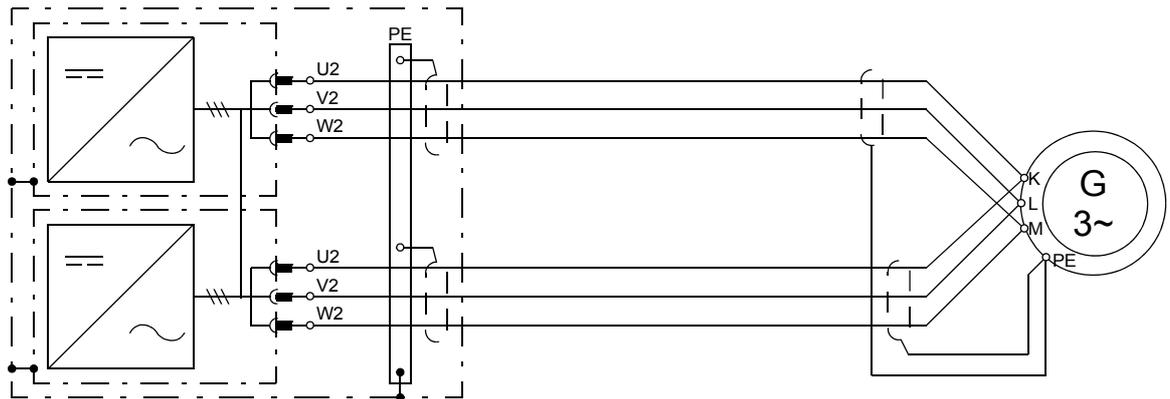
**Note:** Rotor-side cable connection terminals are U2, V2, W2 and PE. To be wired by the user. For selection of the cables, see chapter [Planning the electrical installation](#). For the terminal sizes, tightening torques and lead-throughs, see chapter [Technical data](#).
