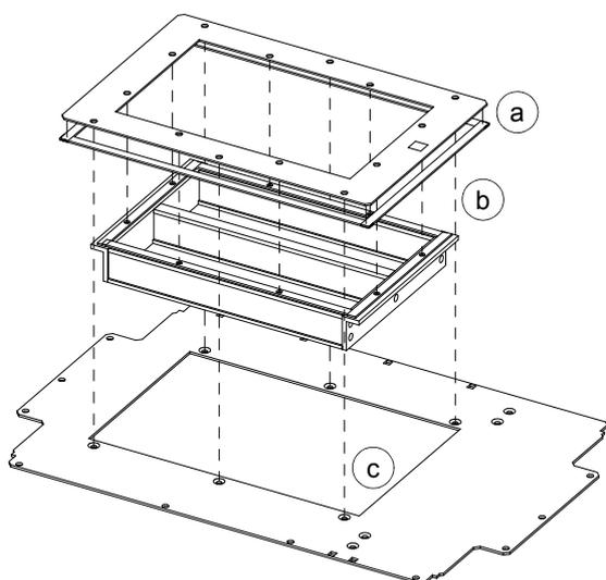
*Fasten the gasket to the collar plate (a).*
