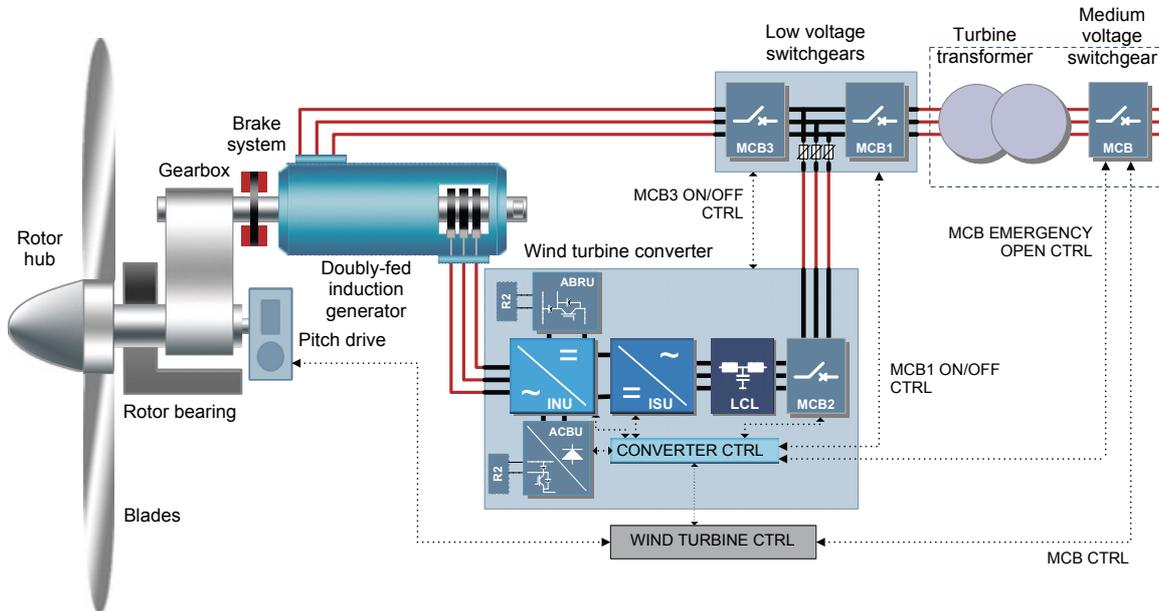
■ **Wind turbine system with medium voltage stator (> 1000 V)**
