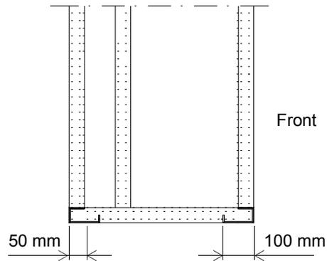
Minimum widths for the floor support (side view)
