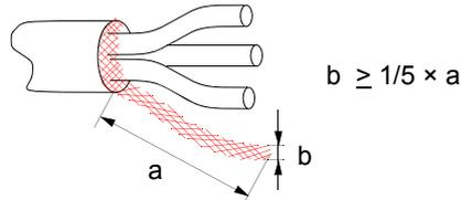
⑥ *Cable lead-through when shielded cable is used*
