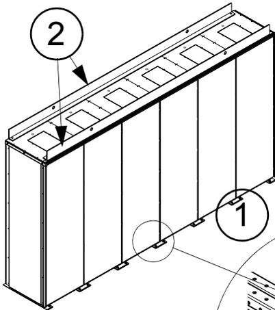
1. Bolt the cabinet to the floor through the holes in each flat bar at the base of the cabinet using M10 or M12 screws.
