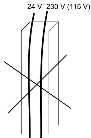
Not allowed unless the 24 V cable is insulated for 230 V (115 V) or insulated with an insulation sleeving for 230 V (115 V).
