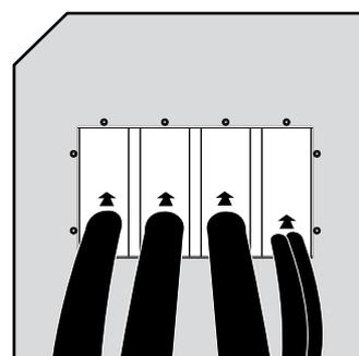
*Route all cables. It is recommended to seal cables at the bottom of the frame and put spare modules on top.*
