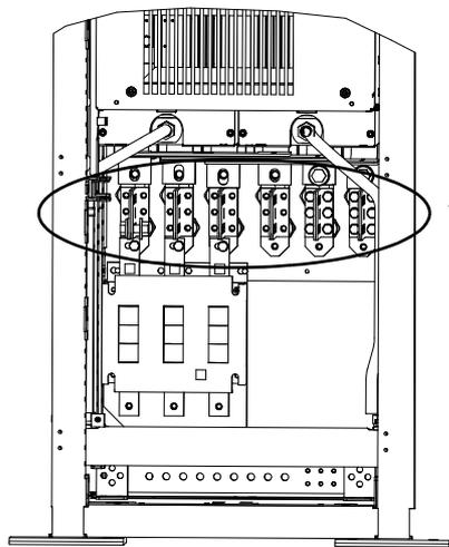
Rotor-side cable connection terminals
