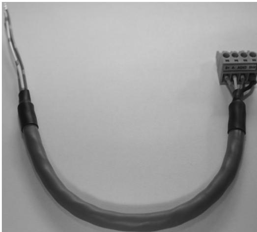
The BACnet MS/TP cable provides connection to the drive's MS/TP connector on terminals 29, 30 and 31. The cable is pre-configured and does not need to be changed.
