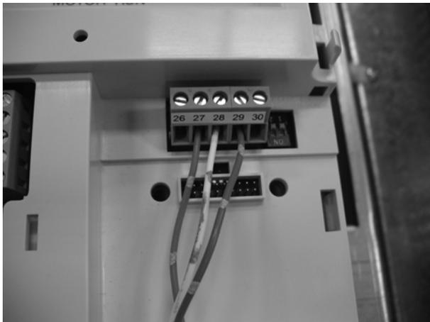
9. For E-Clipse Bypass installations the supplied MS/TP network cable is not long enough. Remove the orange plug from the MS/TP network cable. Replace the cable with Belden 9842 or equivalent. Cut the cable to length and wire to the X1 terminal of E-Clipse as shown in the figure and table.
