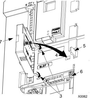
**NOTE!** Correct installation of the ground lead is essential for fulfilling the EMC requirements and for proper operation of the module.
