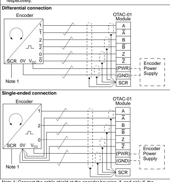
Note 1: Connect the cable shield at the encoder housing, if, and only if, the encoder is isolated from the motor, and from ground.
