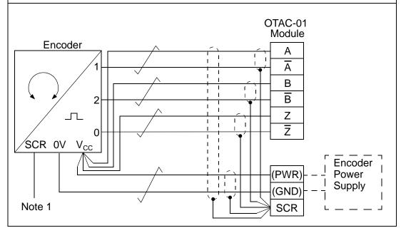
Note 1: Connect the cable shield at the encoder housing, if, and only if, the encoder is isolated from the motor, and from ground.
