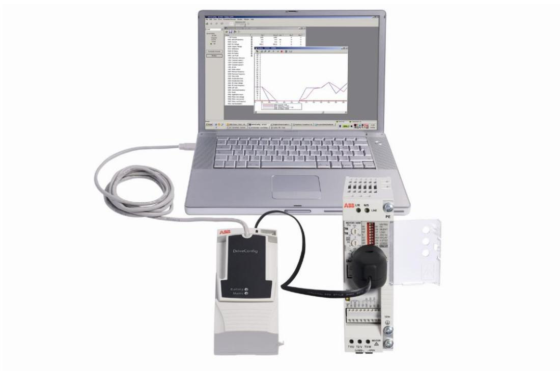
*Figure 3. Connecting the drive using the USB port of the PC (RFDT-02)*
