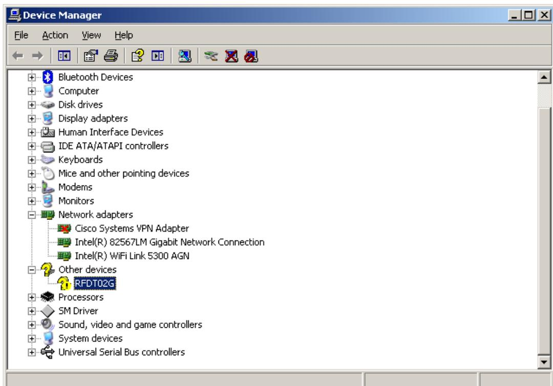
Click left mouse button on the faulty device and select **Properties**. If the device is not working correctly, click **Reinstall driver**. Drivers can be found in the DriveConfig installation folder. Default is C:\Program Files \DriveWare\ DriveConfig\ RFDT-02 Drivers\.
