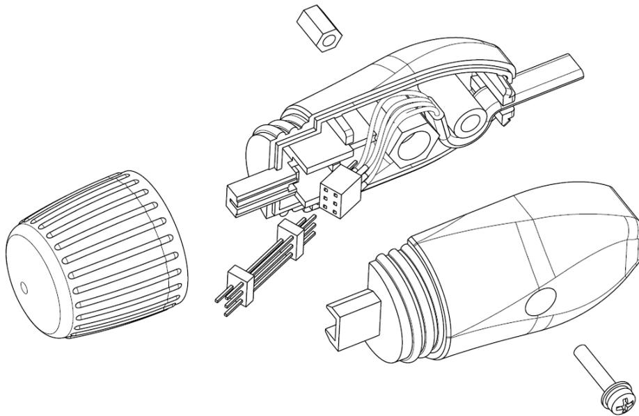
*Figure 2. Replacing the spare pin header*
