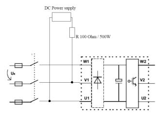
Note! Markings for drive input differs between drive types:
