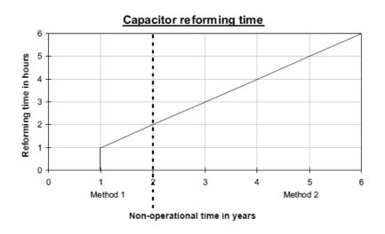
Figure 1. Capacitor reforming time.
