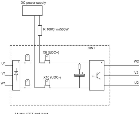
\* Note: IGBT and input bridge not assembled on board
