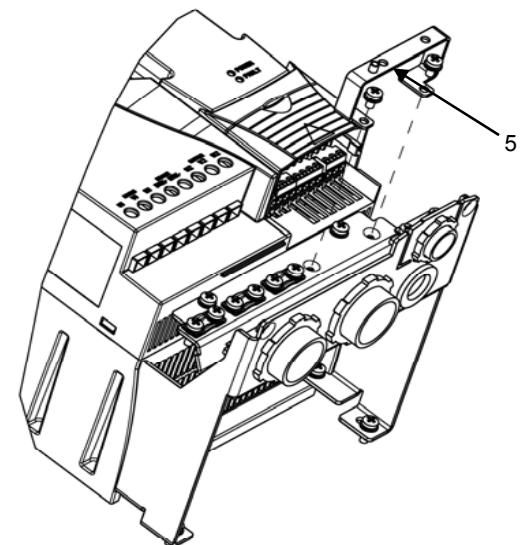
5. With any fieldbus option module except FRSA-00, install the option grounding plate to the gland box frame. See *Mechanical installation* in the drive manual.
