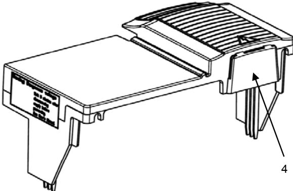
4. If control cables or fieldbus option modules will be installed, remove the detachable lid (4) from the gland box cover.
