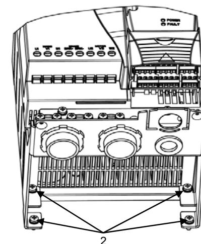
2. Fasten the gland box frame to wall with four M4 screws (not included).
