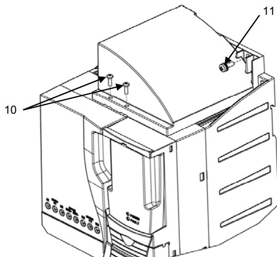
10. Fasten the hood to drive with two M3×12 screws.
