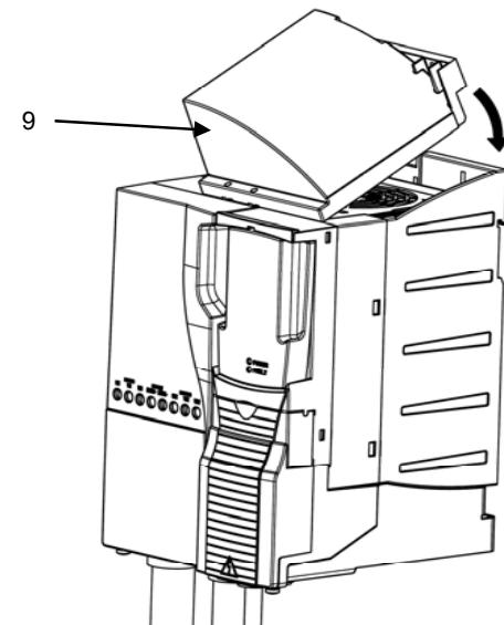
9. Install the hood. First position the front edge carefully, then press the hood downwards until it snaps on.
