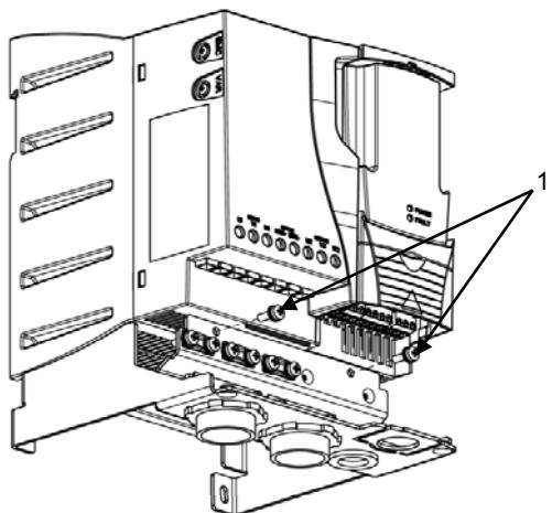
1. Fasten the gland box frame to drive with two M4×12 screws.
