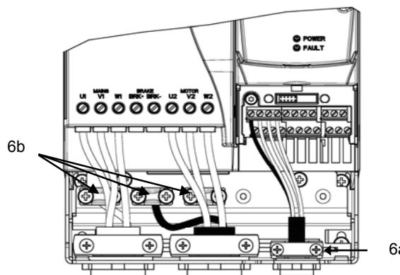
6. Install the clamp (6a) for the control cable, or if cables are run in conduits, replace all clamps with suitable glands (not included). Run cables through the clamps and tighten. Strip cable ends. Fasten the grounding conductor (PE) of the input power cable and the twisted shield of motor cable under the grounding clamps (6b). Connect the conductors to appropriate terminals. See *Electrical installation* in the drive manual.
