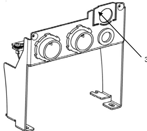
3. If using FPBA-01 or FCAN-01 option module, remove part from gland box frame by bending it.
