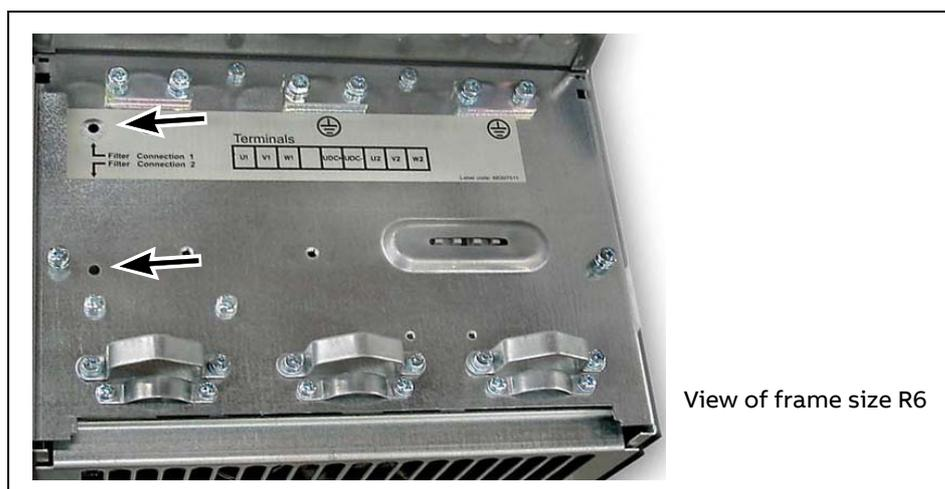
**Note:** When the capacitors of EMC filter +E202 are disconnected, the EMC Directive requirements may not be fulfilled in first environment, but are fulfilled in the second environment.
