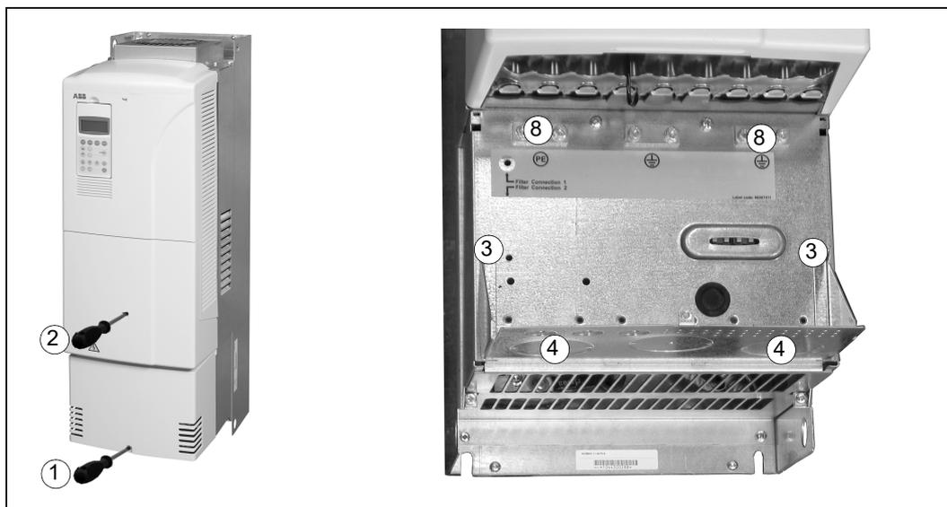
3. Remove the gland plate by undoing the fastening screws.
