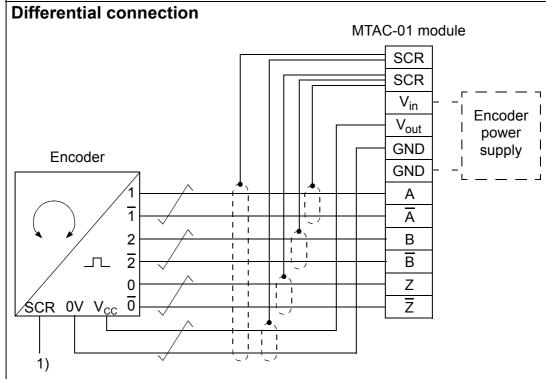
1) Connect the cable shield at the encoder housing, if, and only if, the encoder is isolated from the motor, and from the ground.
