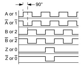
Diagrams show normal phasing: Pulse A/1 leads (i.e. rises earlier than) pulse B/2.
