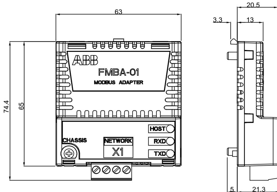
**Mounting:** Into the option slot on the drive
