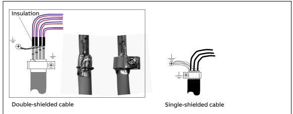
When the outer surface of the shield is covered with non-conductive material:
