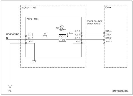
This circuit diagram shows how the AGPS-11 kit is installed.
