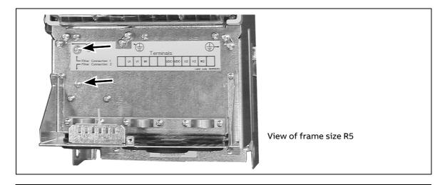
**Note**: When the capacitors of EMC filter +E202 or +E200 are disconnected, the EMC Directive requirements in the second environment are not fulfilled. See *CE marking* (page 132).
