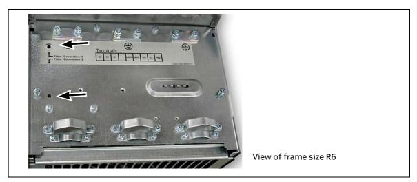
**Note:** When the capacitors of EMC filter +E202 are disconnected, the EMC Directive requirements may not be fulfilled in first environment, but are fulfilled in the second environment.
