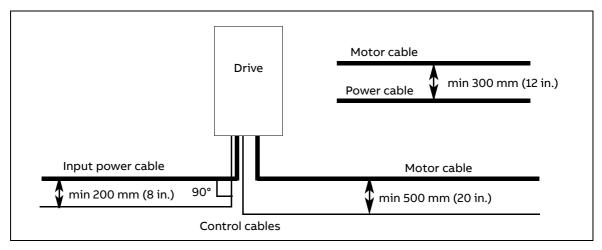
A diagram of the cable routing is shown below.
