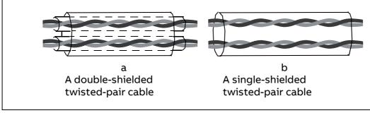
Run analogue and digital signals in separate, shielded cables.
