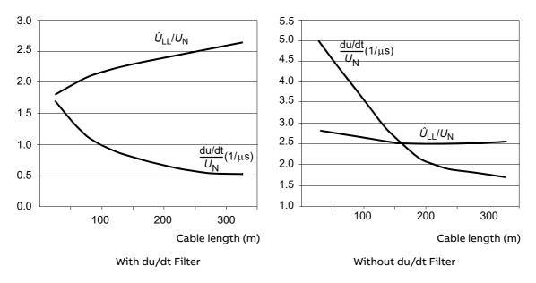
**Note 10:** Sine filters protect the motor insulation system. Therefore, du/dt filter can be replaced with a sine filter. The peak phase-to-phase voltage with the sine filter is approximately  $1.5 \times U_{\rm N}$ .
