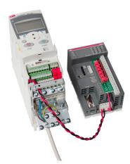
The AC500-eCo can be supplied for testing purpose from the ACS355 drive.
