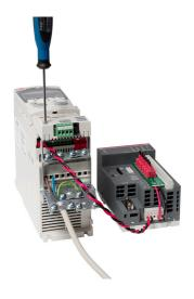
9 Install the Modbus adapter module FMBA-01 and attach the grounding screw.
