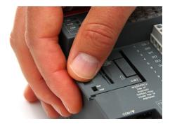
Remove the cover for installation of the accessories.
