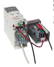
10 Connect the TK505 cable between the AC500-eCo and the FMBA-01 module.
