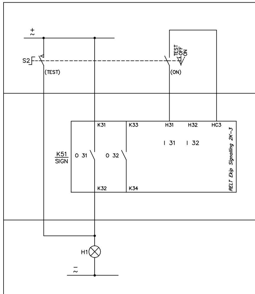
SCHEMA APPLICATIVO PER INTERRUOTTORE EMAX 2 CON MODULO RELT
