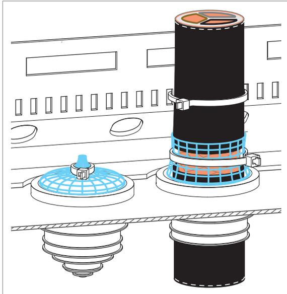
9. Connect the twisted shields of the cables to the PE busbar of the cabinet.
