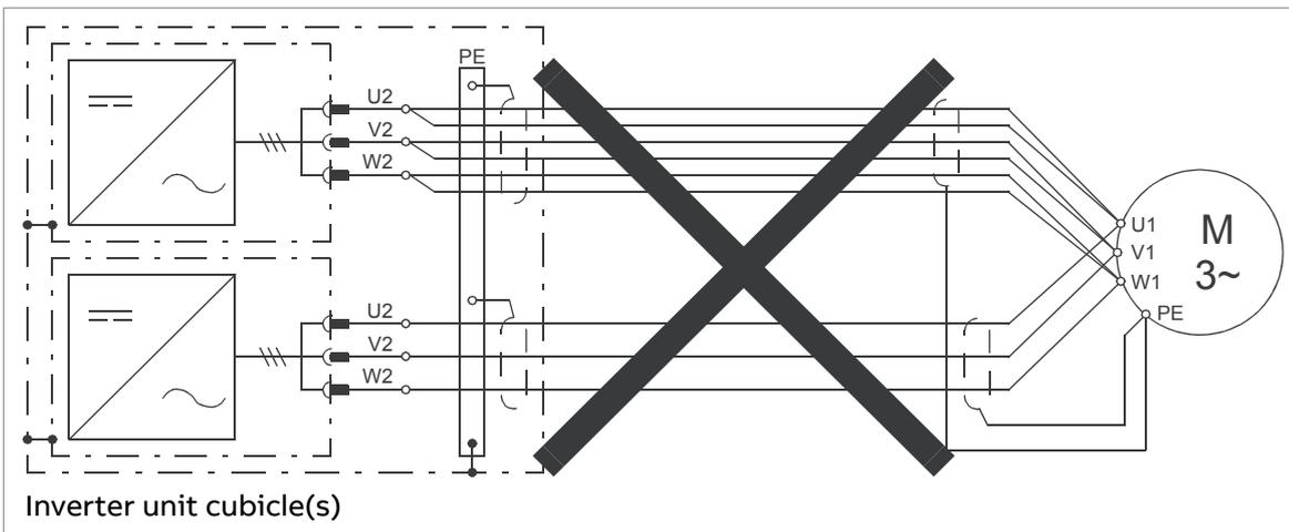
■ **Motor connection diagram (with option +H366)**
