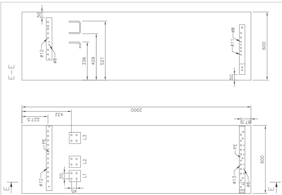
■ Units with main breaker (1000 mm), top cable entry
