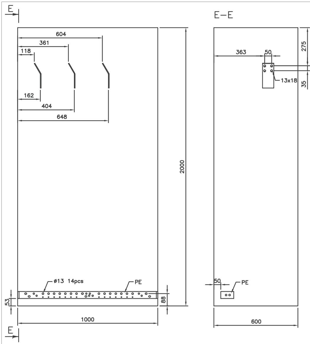
■ Units with common motor terminal cubicle (+H359)
