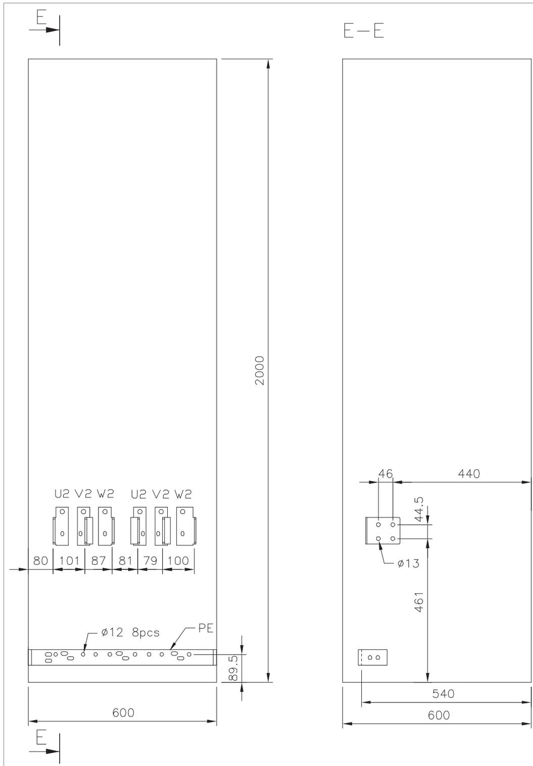
**Inverter module cubicle with two R8i modules, top cable exit**
