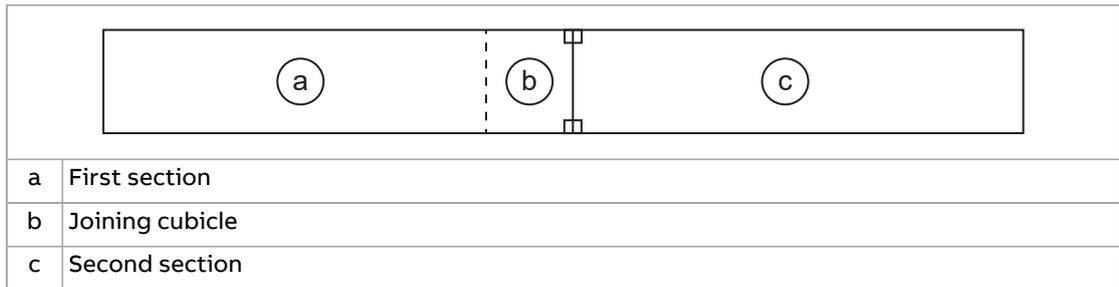
4. Attach the front and rear posts of the joining cubicle to the posts of the other section with 16 screws (8 per post). Tighten the screws to 5 N·m (3.7 lbf·ft).
