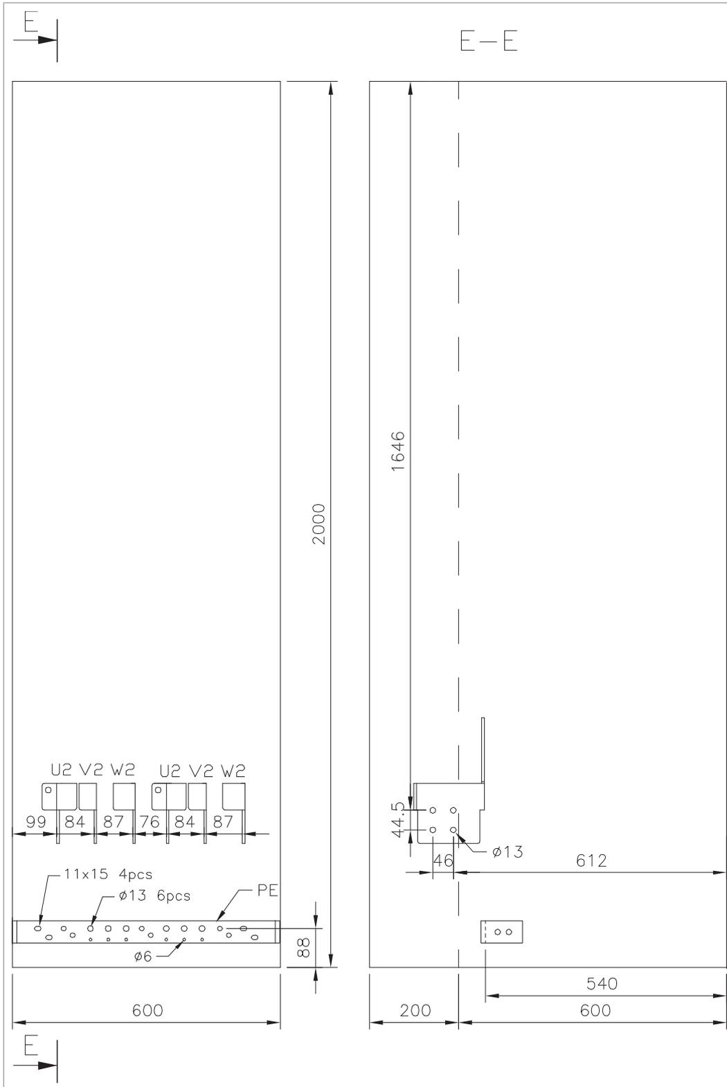
**Inverter module cubicle with three R8i modules, bottom cable exit**
