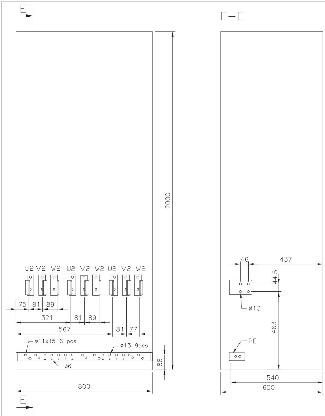
**Inverter module cubicle with three R8i modules, top cable exit**
