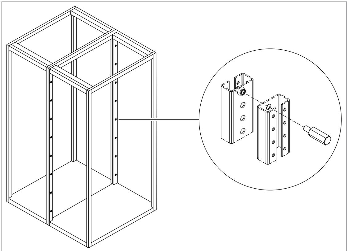
5. Attach the second section to the floor.
