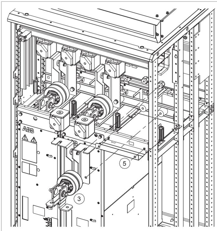
6. If the inverter control unit (A41) is powered from the faulty module, connect the power supply wiring to another module using the extension wire set included.
