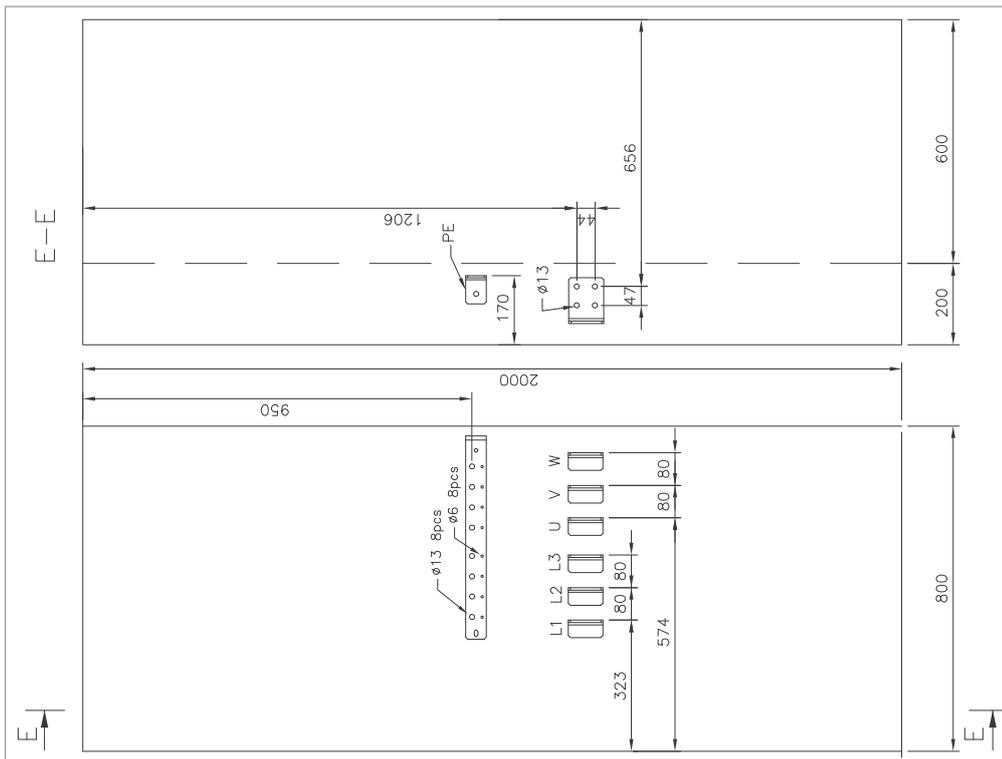
■ **Frame 2×R8i+2×R8i with main switch/disconnector (400 mm), bottom cable entry (+H353)**
