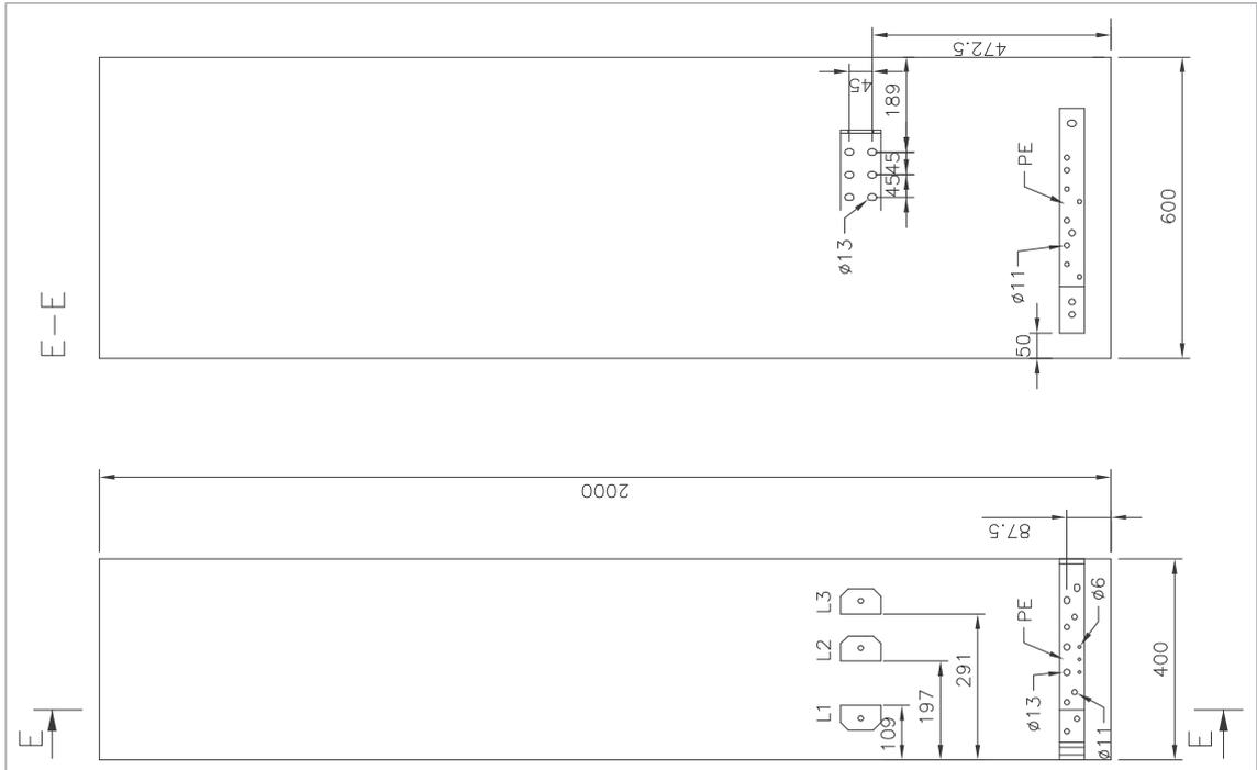
■ **Frame 2×R8i+2×R8i with main switch/disconnector (600 mm), bottom cable entry**
