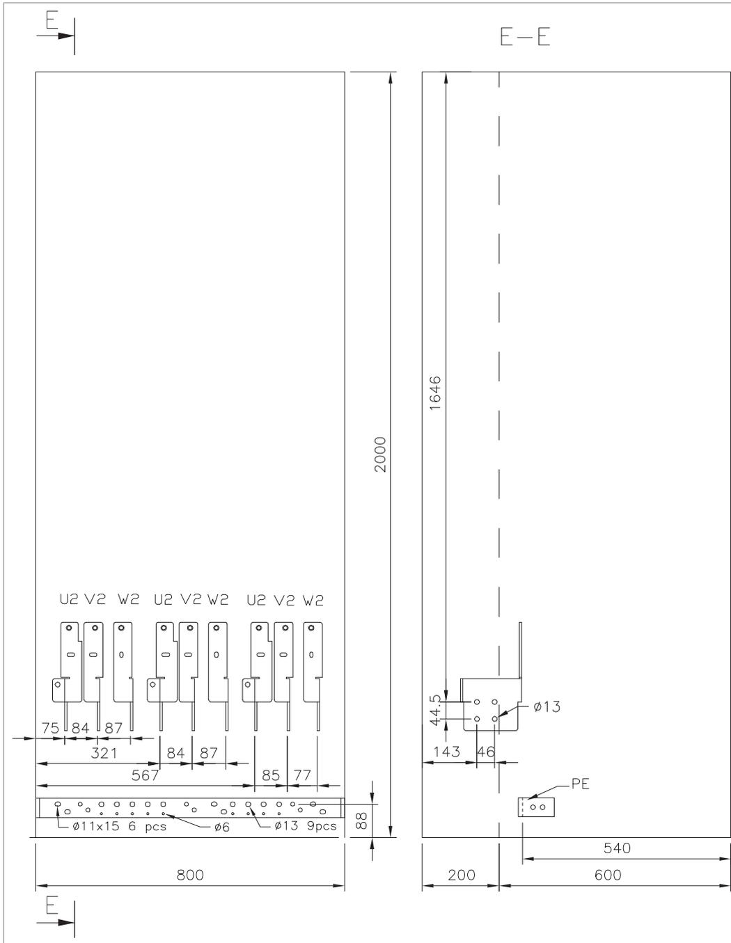
Sine filter cubicle, 1000 mm, bottom cable exit
