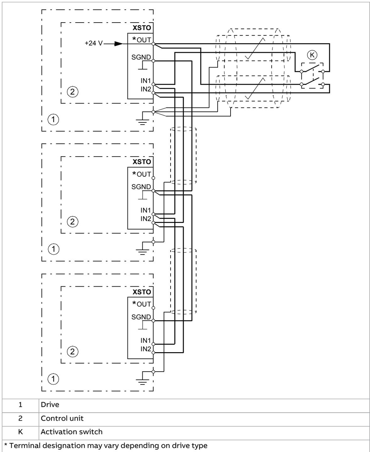
**Internal power supply (example, drives with UCU-2x)**
