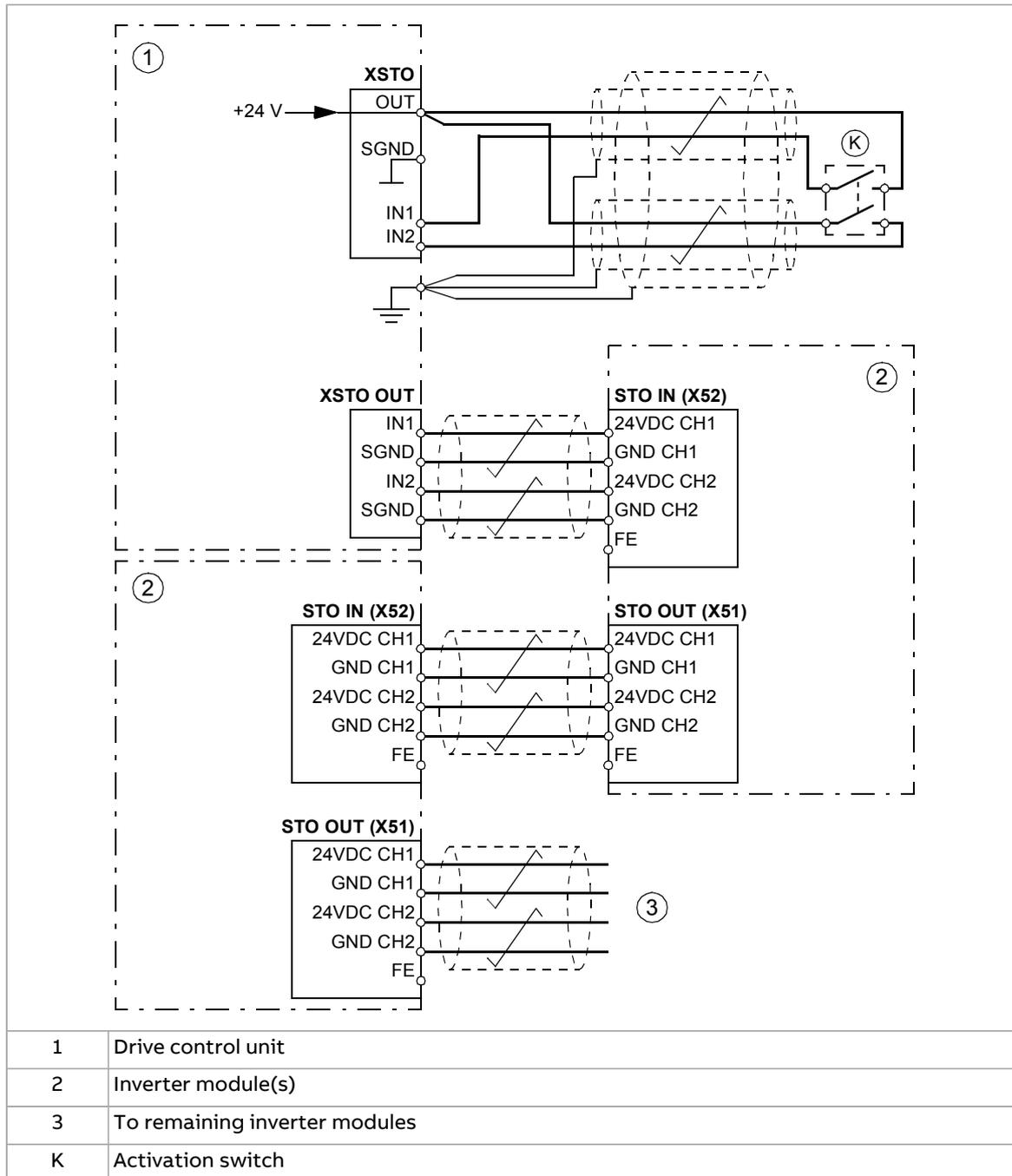
■ Dual-channel connection with internal power supply (UCU-2x)
