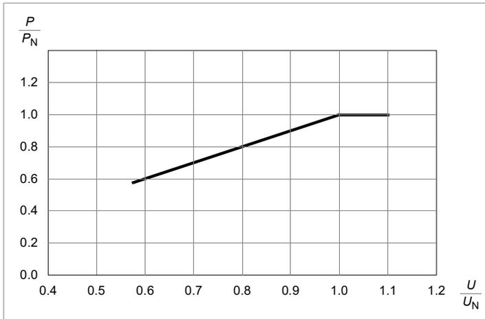
**Example:**  $P_N$  for ACS880-17-1010A-5 is 710 kW. The supply voltage ( $U$ ) is 450 V.  $\rightarrow U / U_N = 450 \text{ V} / 500 \text{ V} = 0.9$ .  $\rightarrow P / P_N = 0.9$   $\rightarrow$  The derated power  $P$  equals  $0.9 \times 710 \text{ kW} = 639 \text{ kW}$ .
