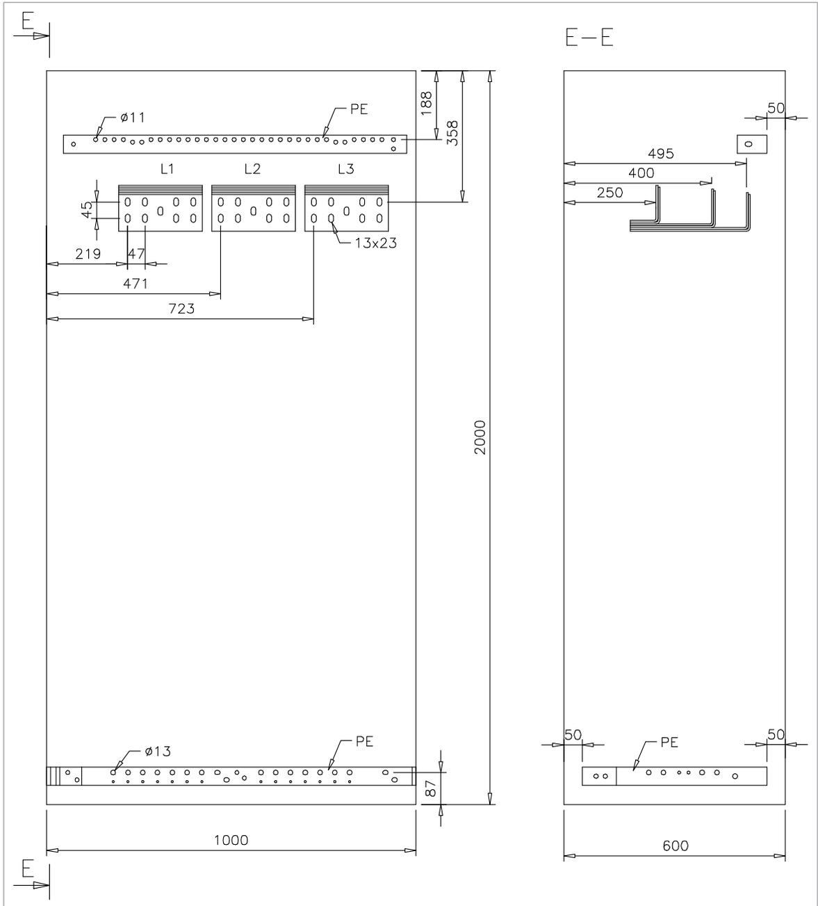
■ **Units with main breaker (1000 mm), bottom cable entry (+H350)**
