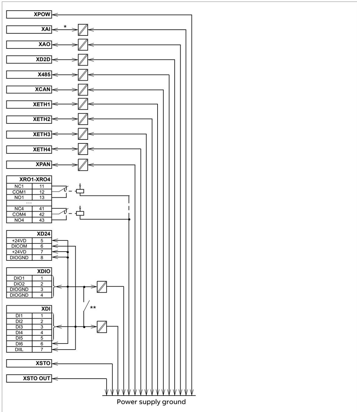
\*The maximum common mode voltage between each AI input and AGND is  $\pm 30$  V
