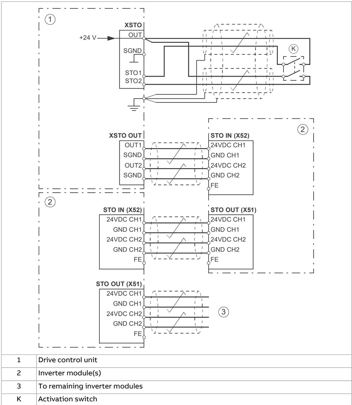
■ **Single-channel connection of activation switch (BCU-x2)**
