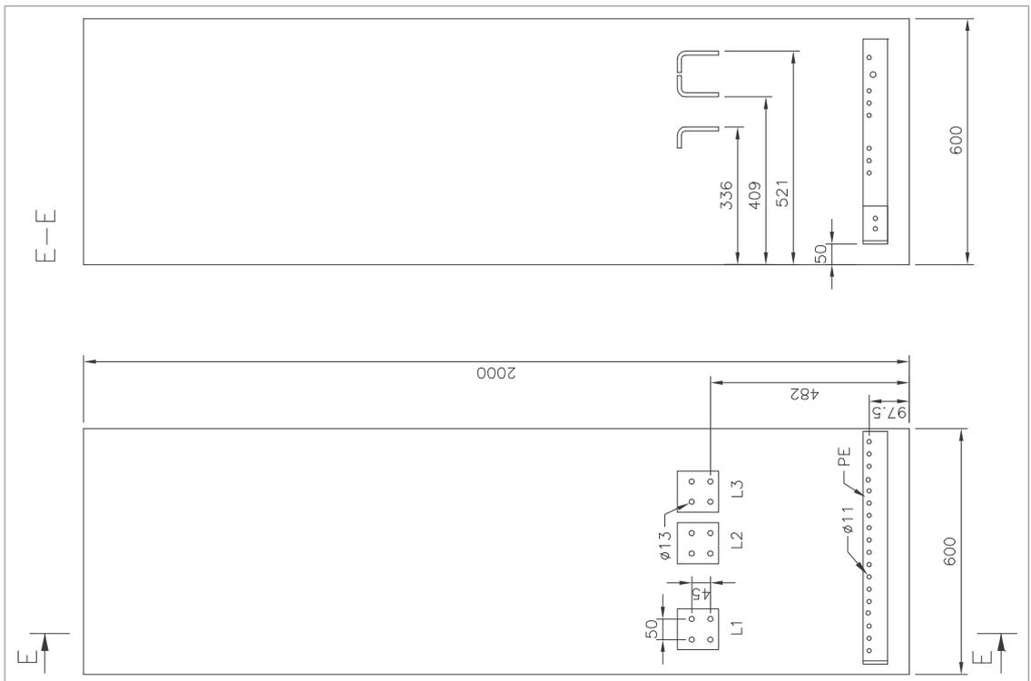
■ Units with main breaker (600 mm, +F255), bottom cable entry
