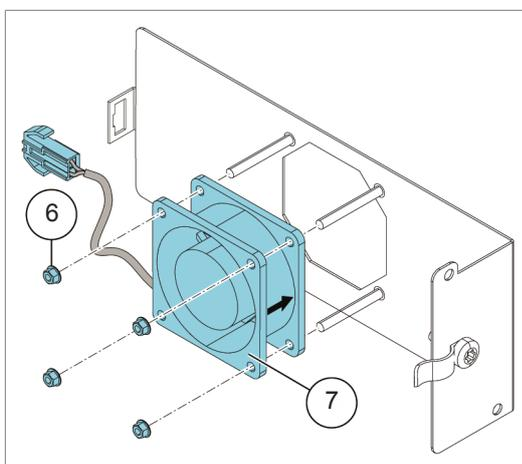
8. Put the fan onto the threaded studs on the fan holder with the airflow direction arrow pointing towards the fan holder.
