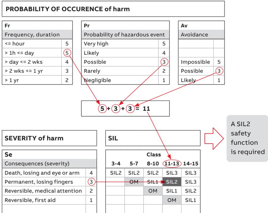
Figure 3-4: Example of SIL assignment table (based on EN/IEC 62061, tables A.1-A.4; A.6)
