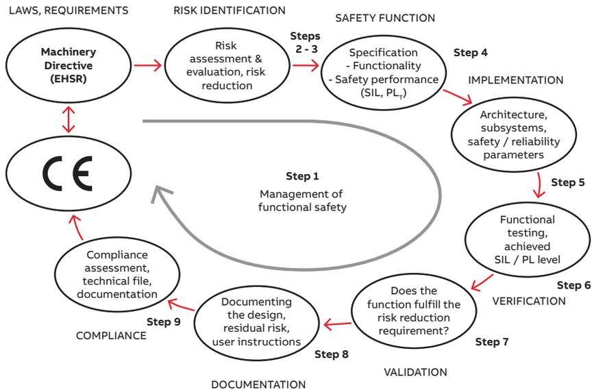
Figure 3-1: Process flow for meeting Machinery Directive requirements
