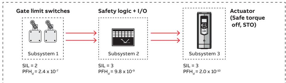
Figure 3-7: Example verification of SIL
