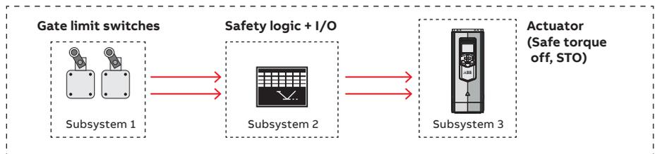
Figure 3-6: Structure of a safety function
