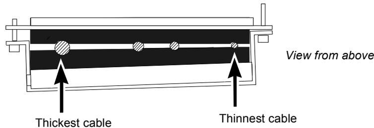
6. If more than one cable go through a grommet, the grommet must be sealed by Loctite 5221 (catalogue number 25551).
