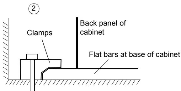
Clamping the cabinet to the floor at the back
