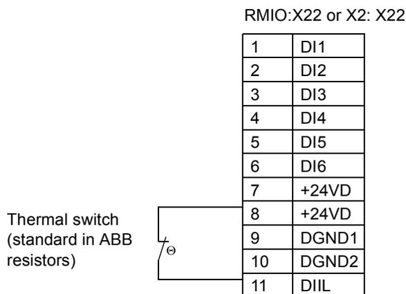
For other control programs, the thermal switch may be wired to a different digital input. Programming of the input to trip the drive by “EXTERNAL FAULT” may be needed. See the appropriate firmware manual.
