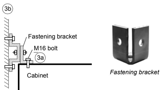
Fastening the cabinet at the top with brackets (side view)
