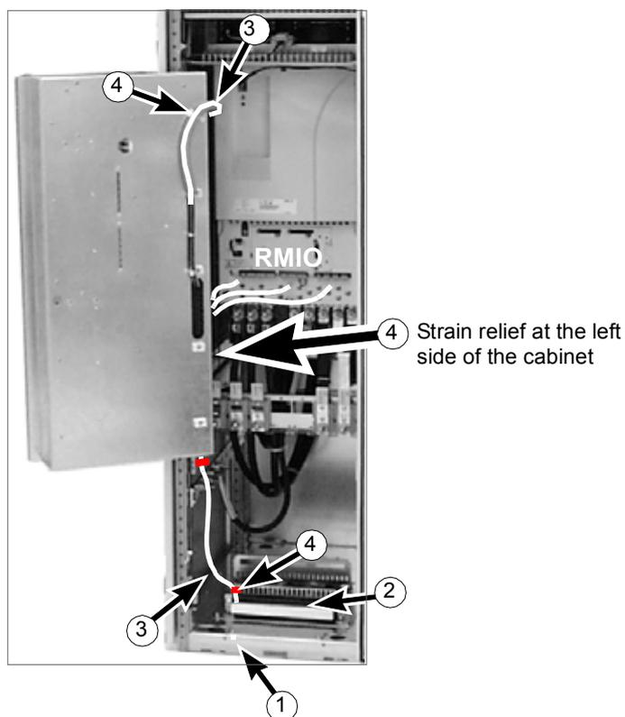
**Routing the cables (frame sizes R7 and R8)**
