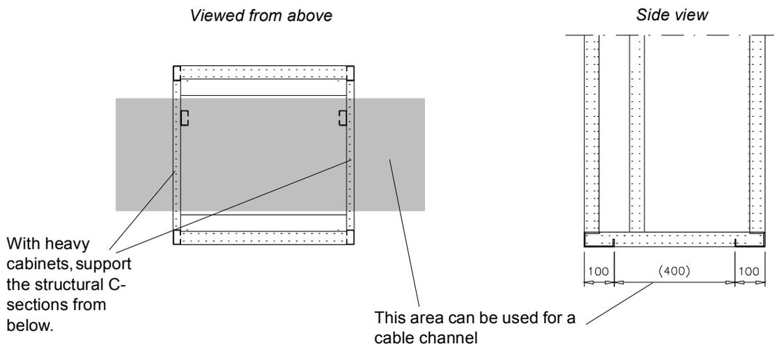
Prevent the cooling air flow from the cable channel to the cabinet by bottom plates. To ensure the degree of protection for the cabinet use the original bottom plates delivered with the unit. With user-defined cable entries take care of the degree of protection, fire protection and EMC compliance.
